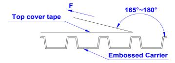
The force for tearing off cover tape is 10 to 130 grams in the arrow direction under the following conditions ( referenced ANSI / EIA - 481 - D - 2008 of 4.11stadnard ).
