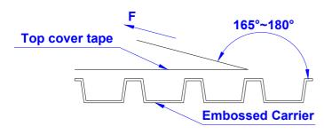
The force for tearing off cover tape is 15 to 80 grams in the arrow direction under the following conditions (referenced ANSI/EIA-481 - D - 2008 of 4.11stadnard ).
