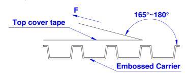
The force for tearing off cover tape is 15 to 80 grams in the arrow direction under the following conditions ( <code>referenced ANSI / EIA - 481 - D - 2008 of 4.11stadnard</code> ).
